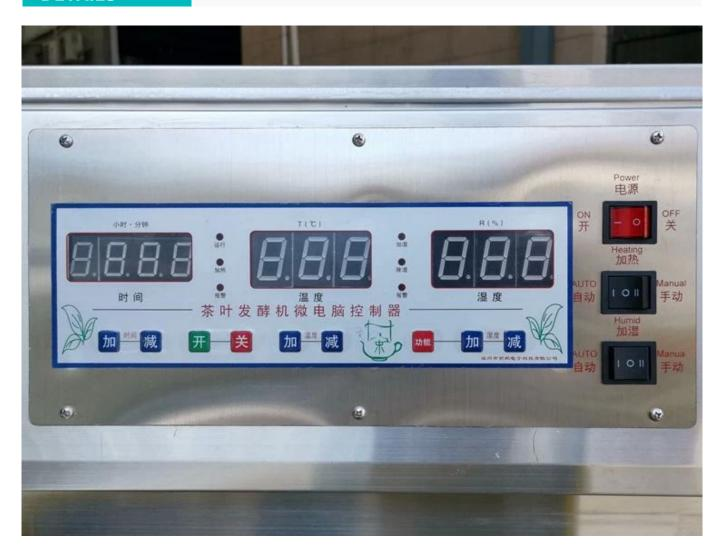
Integrated microcomputer control system, temperature and humidity can be intelligently controlled.
