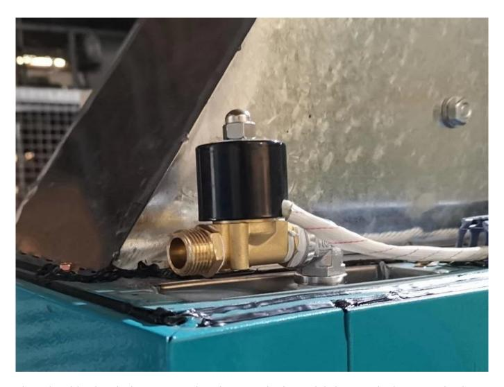
The solenoid valve design ensures that the water in the tank is kept at the best atomization height.
